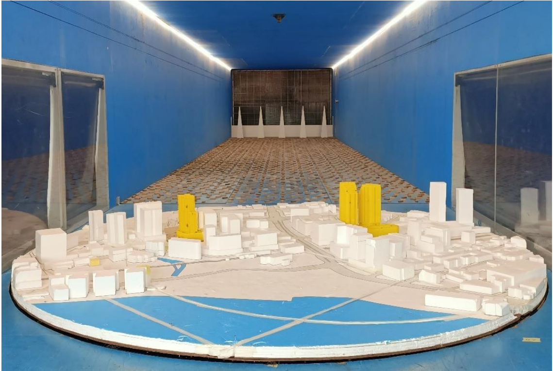
Figure 2b: Photograph of the Wind Tunnel Model Stage 1 Case, view from the north-east
