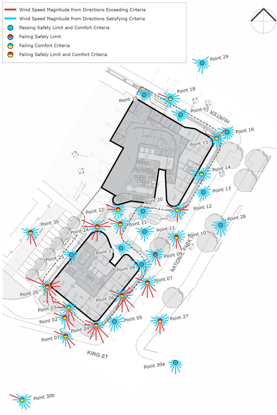
Figure 8a: Wind Tunnel Results – Ground Floor Plan (Stage 2 Case, results shown without treatments applied)
