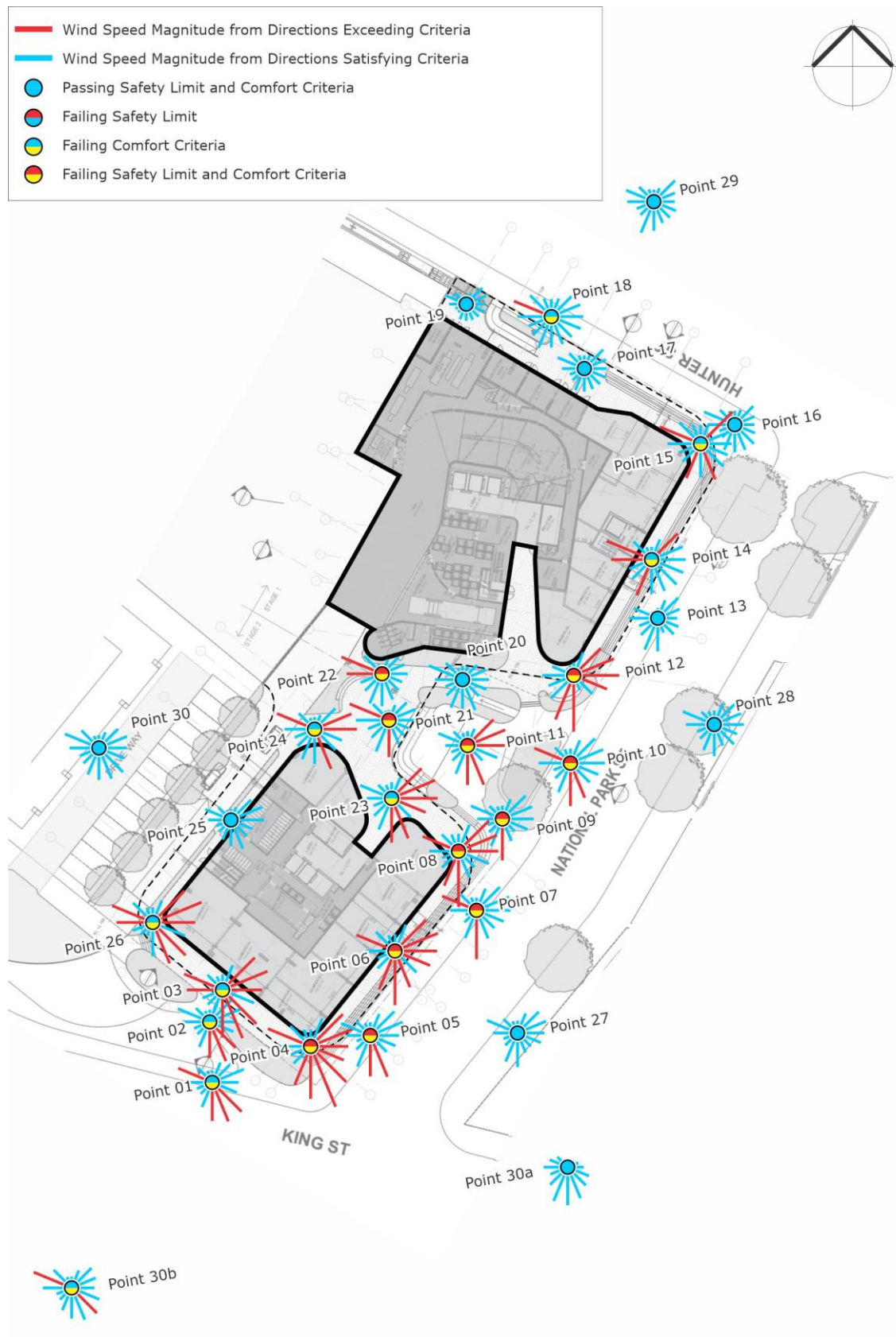
Figure 7a: Wind Tunnel Results – Ground Floor Plan (Stage 1 Case, results shown without treatments applied)
