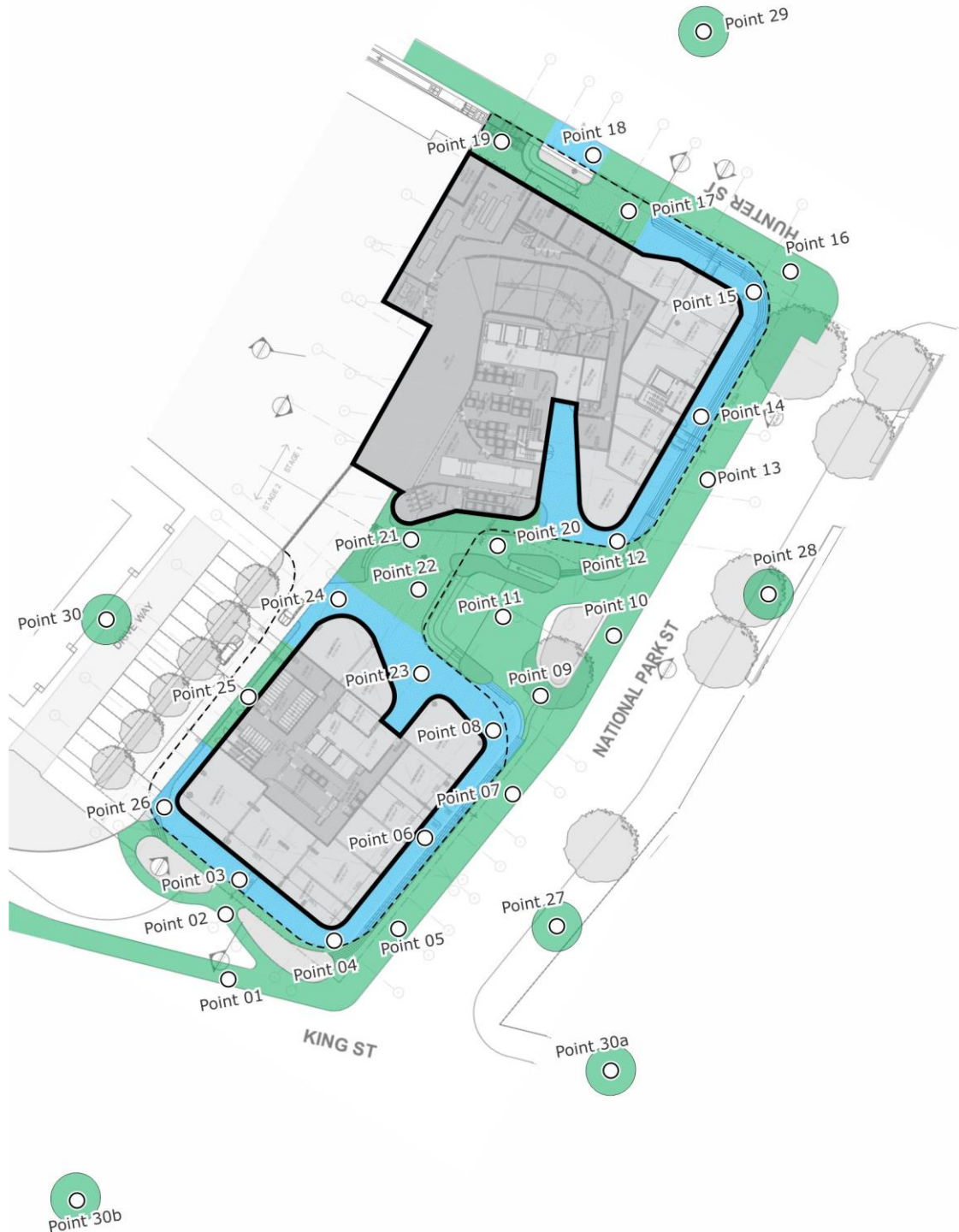
Figure 6a: Study Point Locations and Target Wind Speed Criteria – Ground Floor Plan
