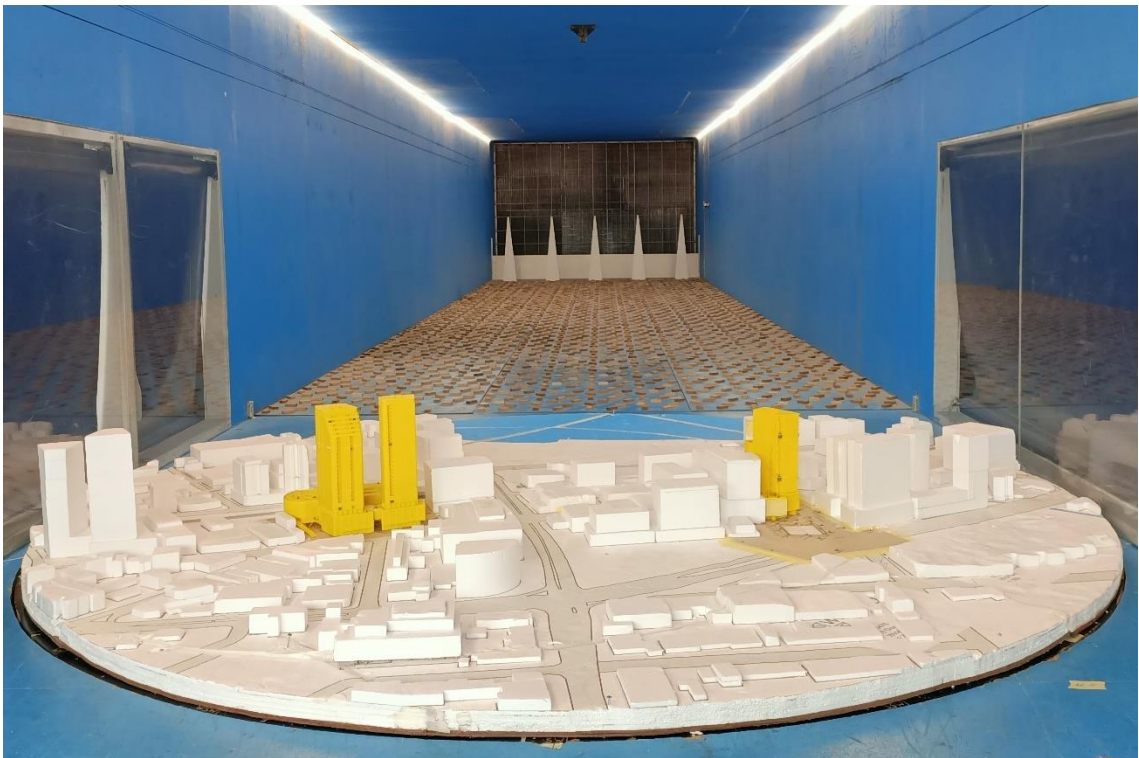
Figure 2e: Photograph of the Wind Tunnel Model Stage 1 Case, view from the south-west
